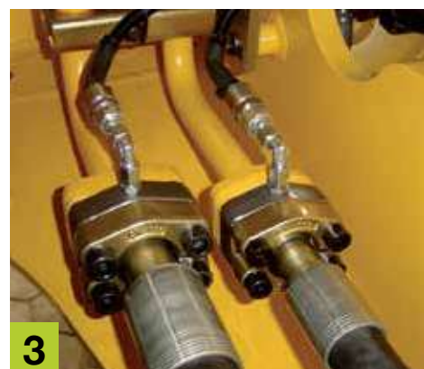
Load sensors installed on the hydraulic circuit of the lifting arms. One sensor is installed on the main pressure side of the lifting cylinder, while the second sensor is installed on the anular side.
